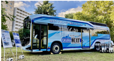
Mobile power generation and supply system "Moving e"
